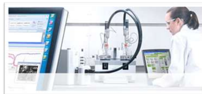
Automated reactor with real-time reaction monitoring
